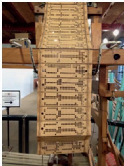
Detail of Jacquard cards at the Museum of Science and Industry Manchester © Hugh Polehampton
